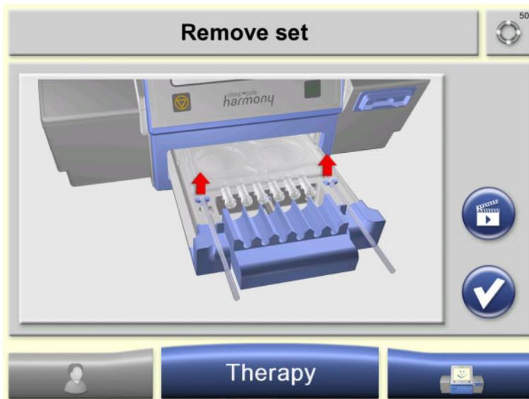
➤ Remove the *sleep-safe Set* from the loading tray. Pull the patient line and the drain line simultaneously upwards until the lines come off the line holders.
