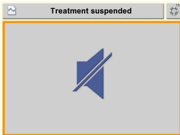
If an initial outflow has been set for the treatment, this message will be displayed when the device detects that the draining of the peritoneal cavity has been completed.
