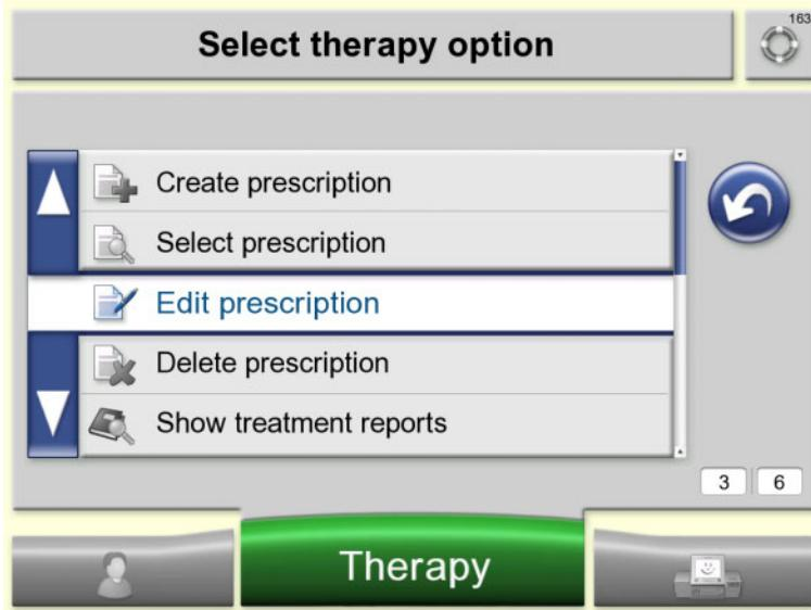
➤ Use the and buttons to move the option **Edit prescription** to the highlighted line in the center. Press on this line to select the option.
