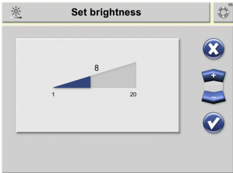
Set the required brightness for the display and all indicator lights (except for the red light of the **status indicator**).
